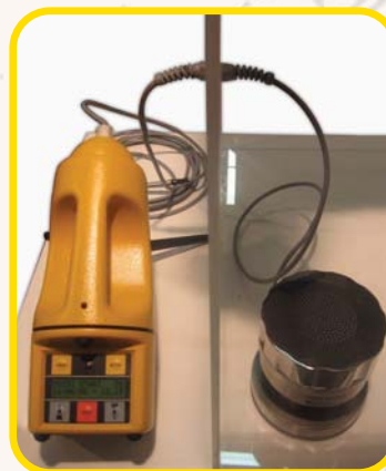
Connection between SAS command unit and aspirating chamber
